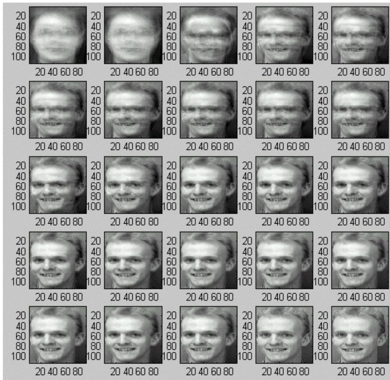
Fig 5 Reconstruction of first image with the number of Eigen Faces
